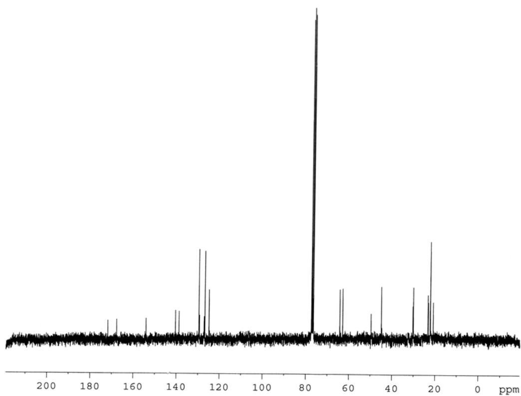
**Fig. 3**  $^{13}\text{C}$  NMR spectrum of MEI in  $\text{CDCl}_3$
