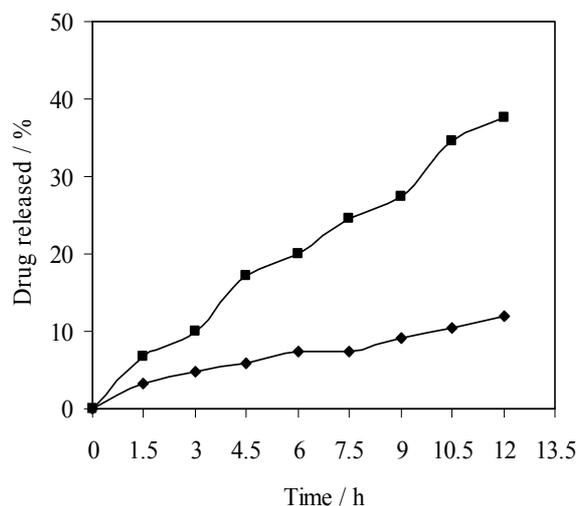
**Fig. 5** Percent of released ibuprofen from polymeric carriers as a function of time at hydrochloric acid buffer (pH 1) and 37 °C. ♦ Poly(MEI-co-BA); ■ Poly(MEI-co-HEMA)
