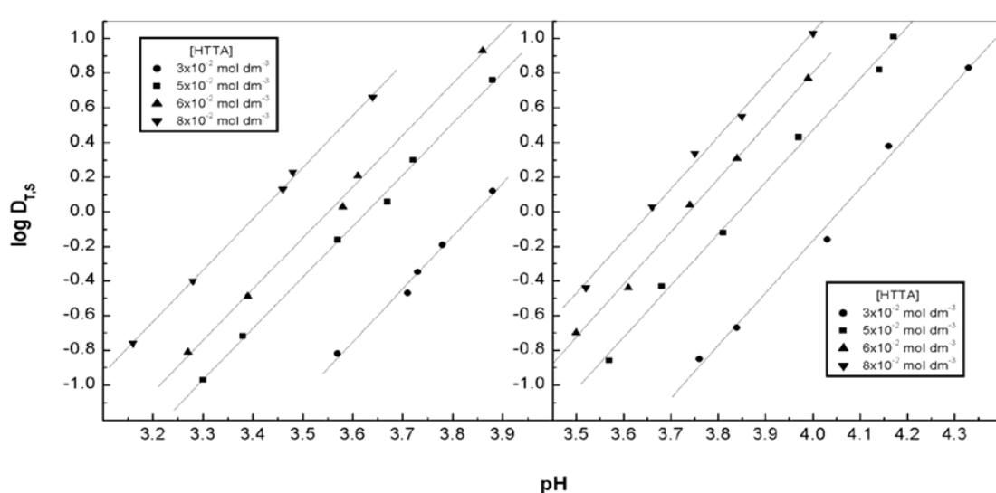
**Fig. 3.**  $\log D_{T,S}$  vs. pH for Gd extraction with HTTA and B15C5 at  $[\text{B15C5}] = 5.10^{-3} \text{ mol} \cdot \text{dm}^{-3}$ . a –  $\text{ClO}_4^-$  medium; b –  $\text{NO}_3^-$  medium.
