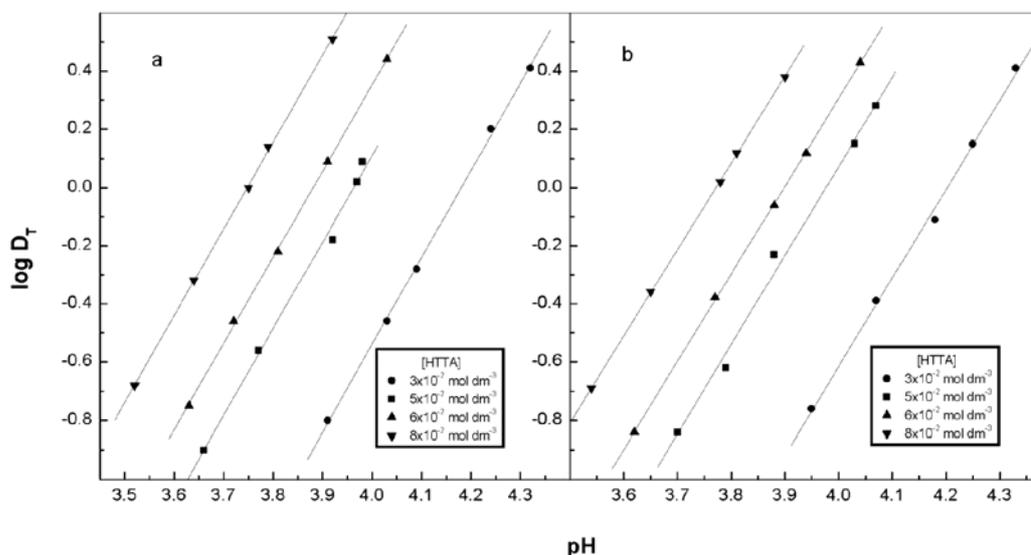
**Fig. 1.** Log  $D_T$  vs. pH for Gd extraction with HTTA in  $C_2H_4Cl_2$ ; a –  $ClO_4^-$  medium; b –  $NO_3^-$  medium.
