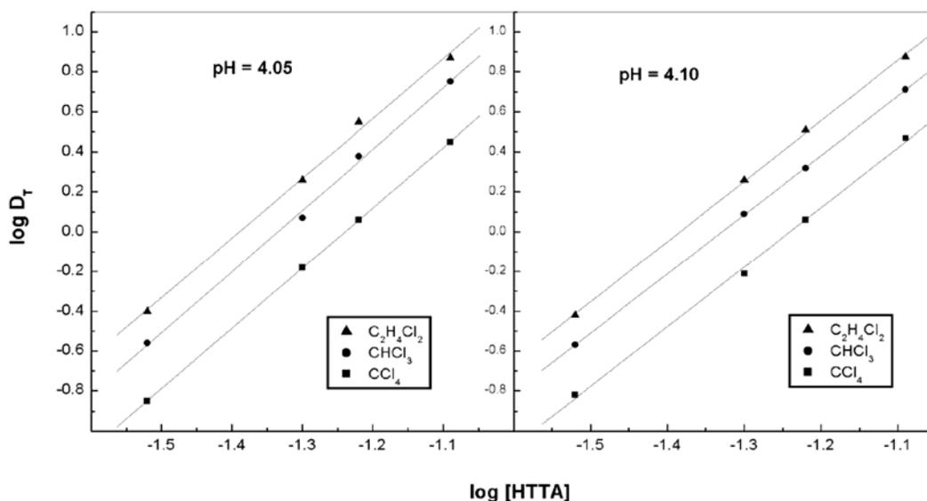
**Fig. 2.** Log  $D_T$  vs. log [HTTA] for Gd extraction. a –  $ClO_4^-$  medium; b –  $NO_3^-$  medium.
