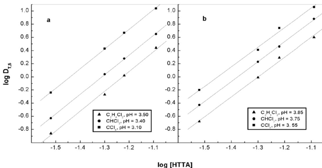
**Fig. 4.**  $\log D_{T,S}$  vs.  $\log [\text{HTTA}]$  for Gd extraction at  $[\text{B15C5}] = 5.10^{-3} \text{ mol} \cdot \text{dm}^{-3}$ . a –  $\text{ClO}_4^-$  medium; b –  $\text{NO}_3^-$  medium.
