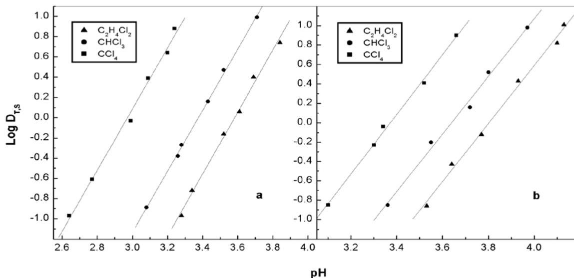
**Fig. 7.**  $\log D_{T,S}$  vs. pH for Gd extraction at  $[HTTA] = 5.10^{-2} \text{ mol.dm}^{-3}$  and  $[B15C5] = 5.10^{-3} \text{ mol.dm}^{-3}$ . a –  $\text{ClO}_4^-$  medium; b –  $\text{NO}_3^-$  medium.
