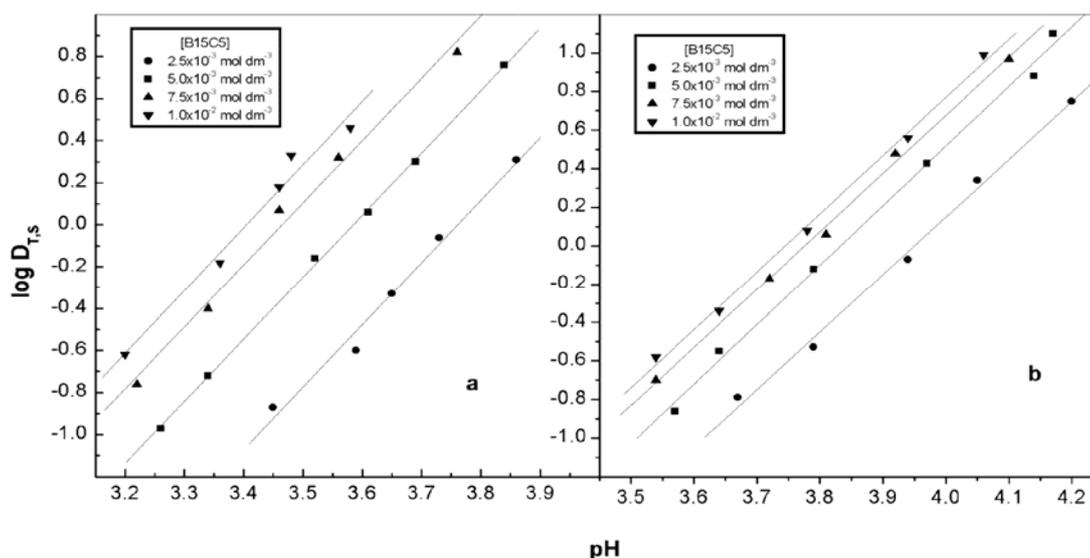
**Fig. 5.** Log  $D_{T,S}$  vs. pH for Gd extraction with HTTA and B15C5 at  $[HTTA] = 5.10^{-2} \text{ mol}\cdot\text{dm}^{-3}$ . a –  $\text{ClO}_4^-$  medium; b –  $\text{NO}_3^-$  medium.
