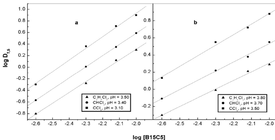
**Fig. 6.** Log  $D_{T,S}$  vs. log  $[B15C5]$  for Gd extraction at  $[HTTA] = 5.10^{-2} \text{ mol}\cdot\text{dm}^{-3}$ . a –  $\text{ClO}_4^-$  medium; b –  $\text{NO}_3^-$  medium.
