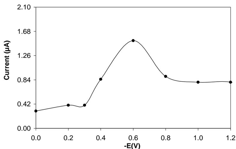
**Fig. 4.** Effect of accumulation potential on DPASV peak current of As(III). Conditions;  $6.0 \mu\text{g mL}^{-1}$  of As(III) concentration,  $0.2 \times 10^{-3} \text{ mol L}^{-1}$  of phenylpiperazine dithiocarbamate; scan rate  $12 \text{ mVs}^{-1}$ ; sodium acetate buffer (pH 4.0); accumulation time 80 Sec.
