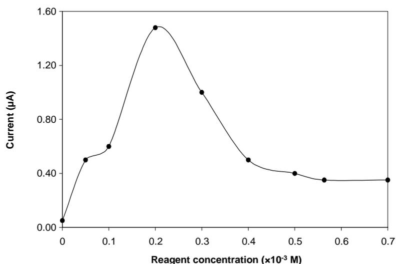
**Fig. 3.** Effect of the reagent concentration on DPASV peak current of As(III). Conditions;  $6.0 \mu\text{g mL}^{-1}$  of As(III) concentration, scan rate  $12 \text{ mVs}^{-1}$ ; accumulation potential  $-0.64 \text{ V}$ , sodium acetate buffer (pH 4.0); accumulation time 80 Sec.
