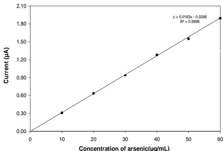
**Fig. 7.** Calibration plot for the DPASV determination of As(III). Conditions;  $0.2 \times 10^{-3}$  mol L<sup>-1</sup> of phenylpiperazine dithiocarbamate; scan rate 12 mV s<sup>-1</sup>; accumulation potential -0.64 V, sodium acetate buffer (pH 4.0); accumulation time 80 Sec.
