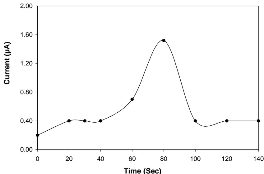
**Fig. 5.** Effect of accumulation time on DPASV peak current of As(III). Conditions;  $6.0 \mu\text{g mL}^{-1}$  of As(III) concentration,  $0.2 \times 10^{-3} \text{ mol L}^{-1}$  of phenylpiperazine dithiocarbamate; scan rate  $12 \text{ mV s}^{-1}$ ; accumulation potential  $-0.64 \text{ V}$ , sodium acetate buffer (pH 4.0).
