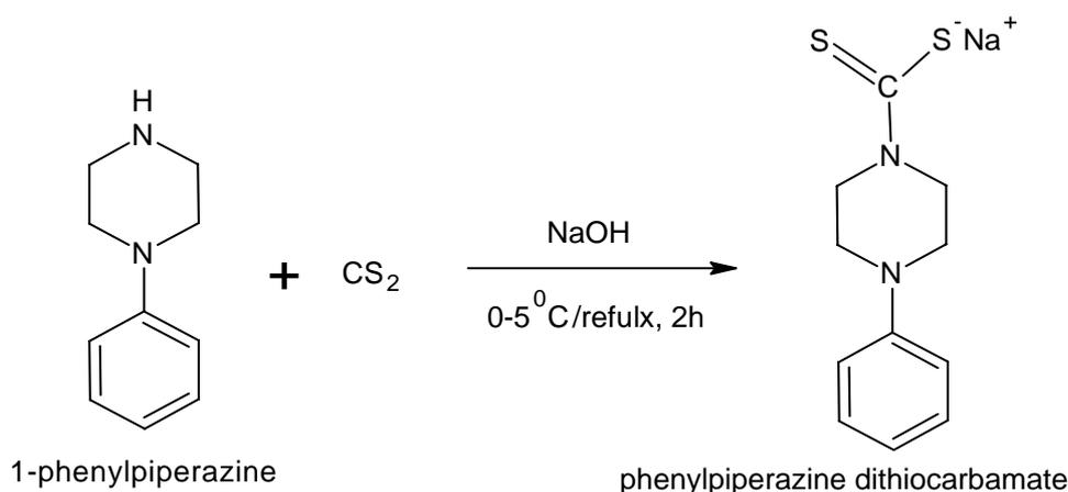
**Scheme 1** Preparation of sodium salts of phenylpiperazine dithiocarbamate.
