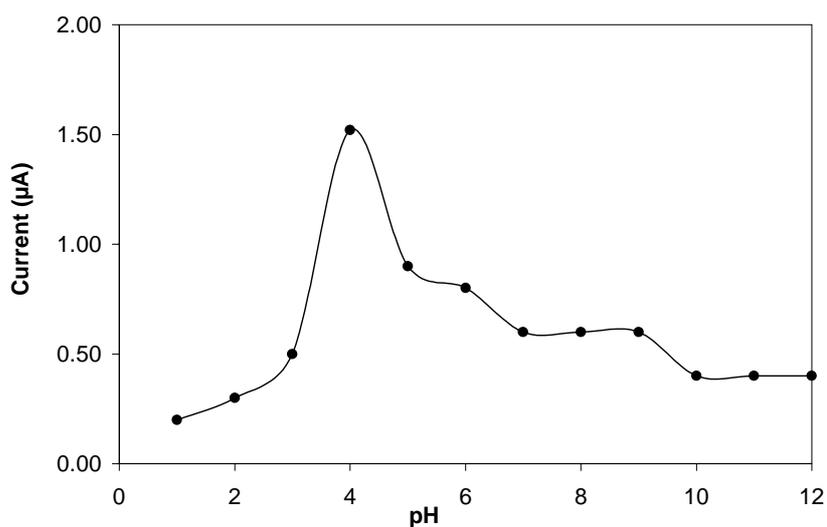
**Fig. 2.** Effect of pH on DPASV peak current of As(III); Conditions;  $6.0 \mu\text{g mL}^{-1}$  of As(III) concentration, accumulation potential -0.64 V, sodium acetate buffer (pH 4.0); accumulation time 80 Sec.
