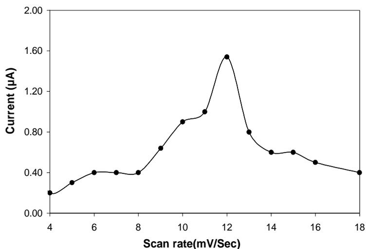
**Fig. 6.** Effect of scan rate on DPASV peak current of As(III); Conditions;  $6.0 \mu\text{g mL}^{-1}$  of As(III) concentration,  $0.2 \times 10^{-3} \text{ mol L}^{-1}$  of phenylpiperazine dithiocarbamate; accumulation potential  $-0.64 \text{ V}$ , sodium acetate buffer (pH 4.0); accumulation time 80 Sec.
