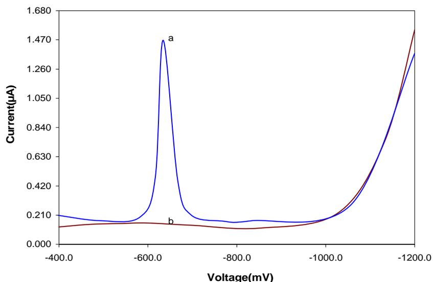
**Fig. 1.** Anodic stripping voltammogram of As(III) peak at -640.0 mV: (a)  $0.2 \times 10^{-3}$  mol L<sup>-1</sup> of phenylpiperazine dithiocarbamate + 0.05 mol L<sup>-1</sup> of sodium acetate buffer (pH 4.0) with experimental conditions (b) blank..
