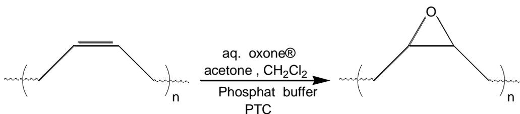
**Scheme 1** Catalytic epoxidation of cis-polybutadiene.
