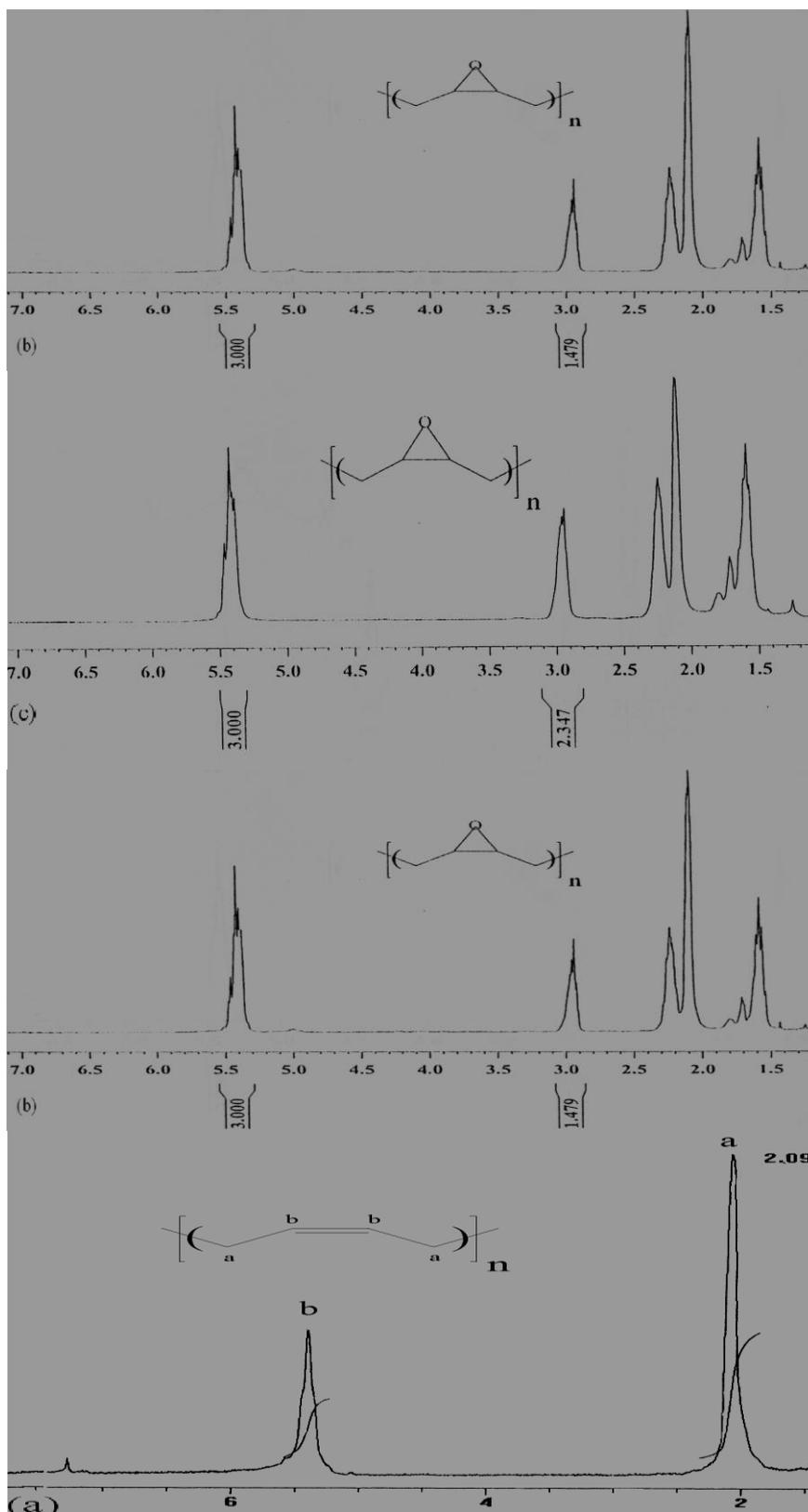
**Fig. 1.**  $^1\text{H}$ NMR spectra of cis-polybutadiene (a) and epoxidized cis-polybutadiene [(b), (c) and (d)]
