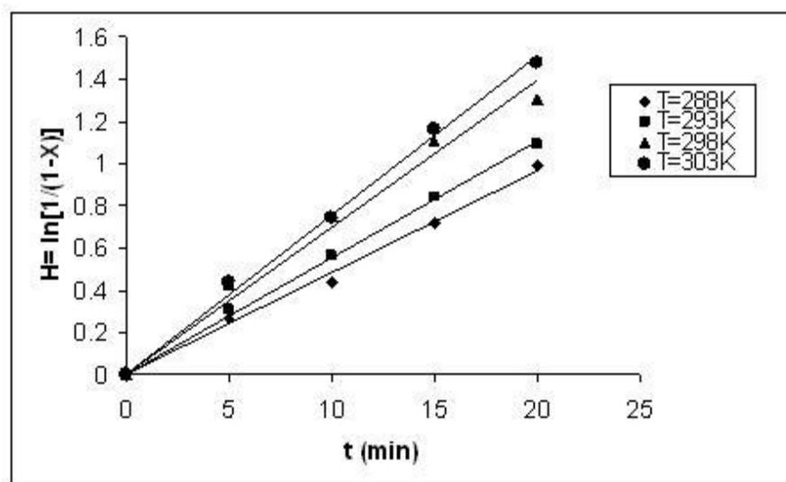
**Fig. 6.** Plot of H vs. reaction time at different temperatures, polymer, catalyst and oxone<sup>®</sup> are 24 g L<sup>-1</sup>, 2.48 mmol L<sup>-1</sup> and 0.079 mol L<sup>-1</sup>, respectively.
