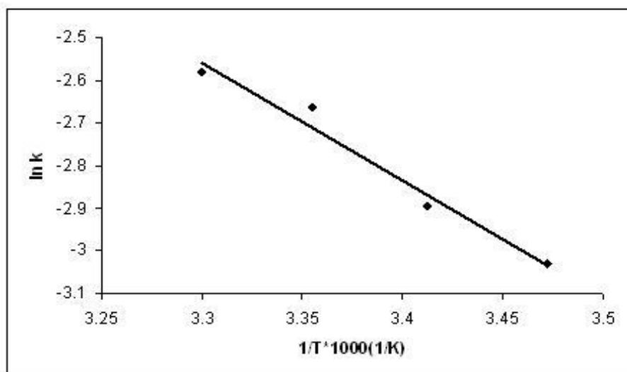
**Fig. 7.** Arrhenius plot of catalytic epoxidation of cis-polybutadiene.
