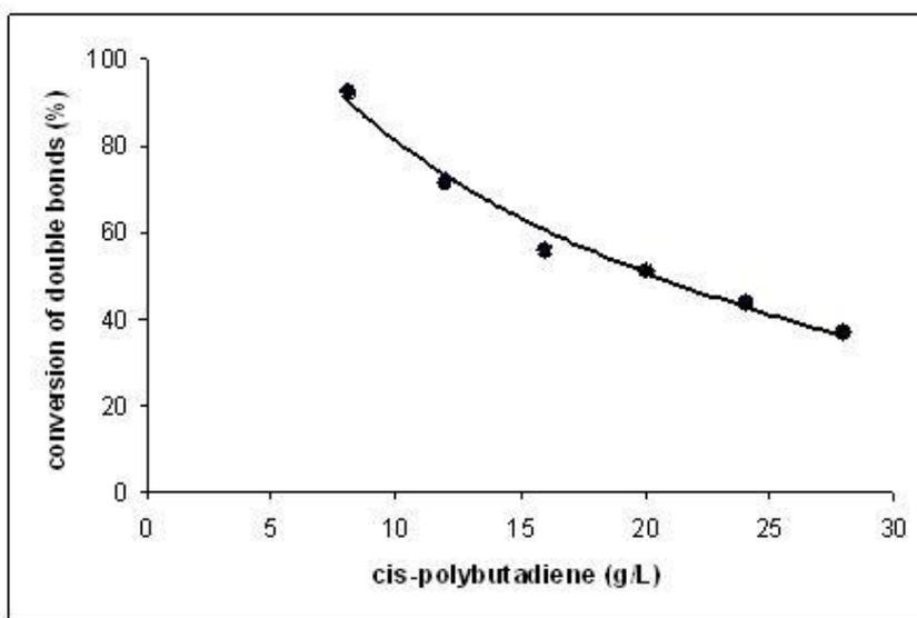
**Fig. 4.** Conversion of double bonds vs. concentration of polymer, oxone<sup>®</sup> and catalyst are 0.079 M and 2.48 mmol L<sup>-1</sup> respectively and reactions were performed at 298 K and 60 min.
