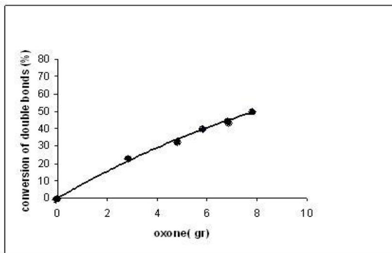
**Fig. 3.** Conversion of double bonds vs. concentration of oxone<sup>®</sup>. Polymer and catalyst are 24 g L<sup>-1</sup> and 2.48 mmol L<sup>-1</sup> respectively and reactions were performed at 298 K and 60 min.
