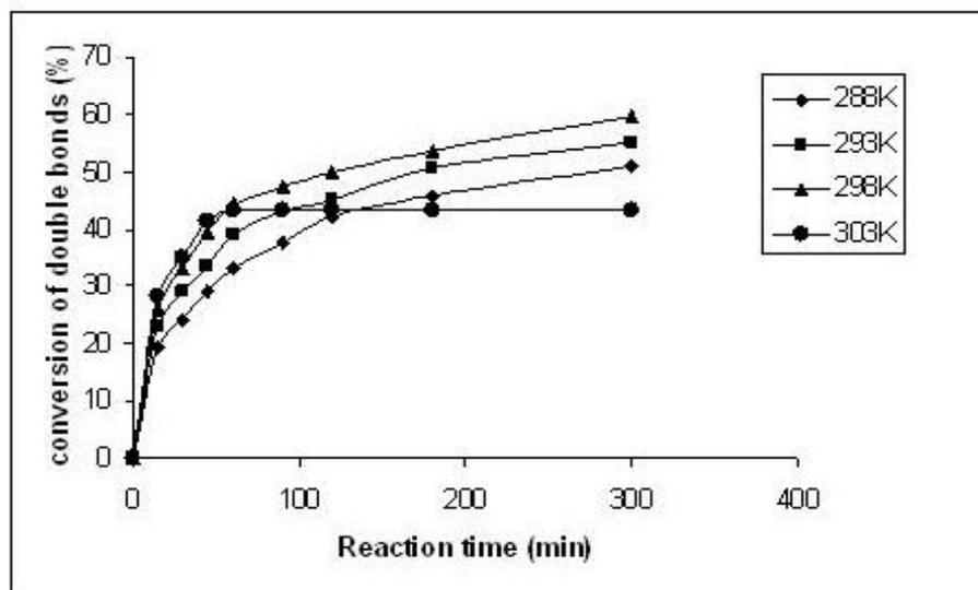
**Fig. 5.** Dependence of double bonds conversion on reaction time at different temperatures, polymer, catalyst, oxone<sup>®</sup> are 24 g L<sup>-1</sup>, 2.48 mmol L<sup>-1</sup>, 0.079 mol L<sup>-1</sup>, respectively.
