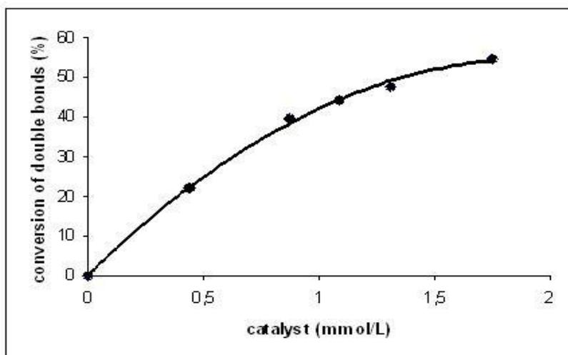
**Fig. 2.** Conversion of double bonds vs. concentration of catalyst, polymer and oxone<sup>®</sup> are 24 g/L and 0.079 M respectively and reactions were performed at 298 K and 60 min.
